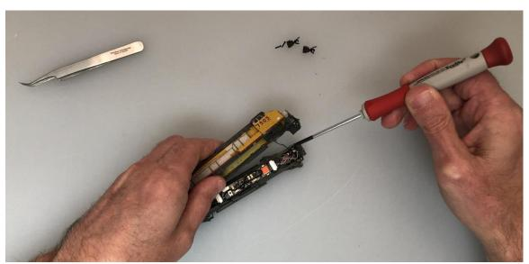
Be aware of the lighting harness that is connected to the cab. You do not want to pull the shell off too fast or with too much force, else these wires can break.
