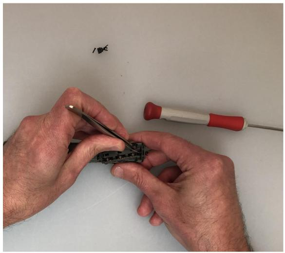
(Hint: You may need to use a set of curved tweezers to pull the screw out. Also, when pulling the coupler out and away from the chassis try to pinch it in a way that will not allow the coupler pocket to come apart. Re-assembly can be difficult)
